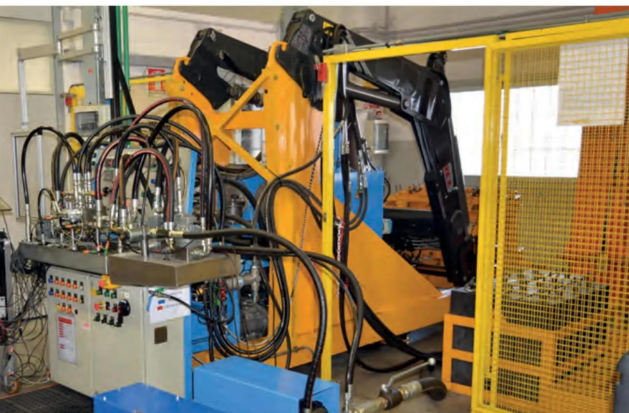
Walvoil front loader test of the EPX system at the Innovation Center
